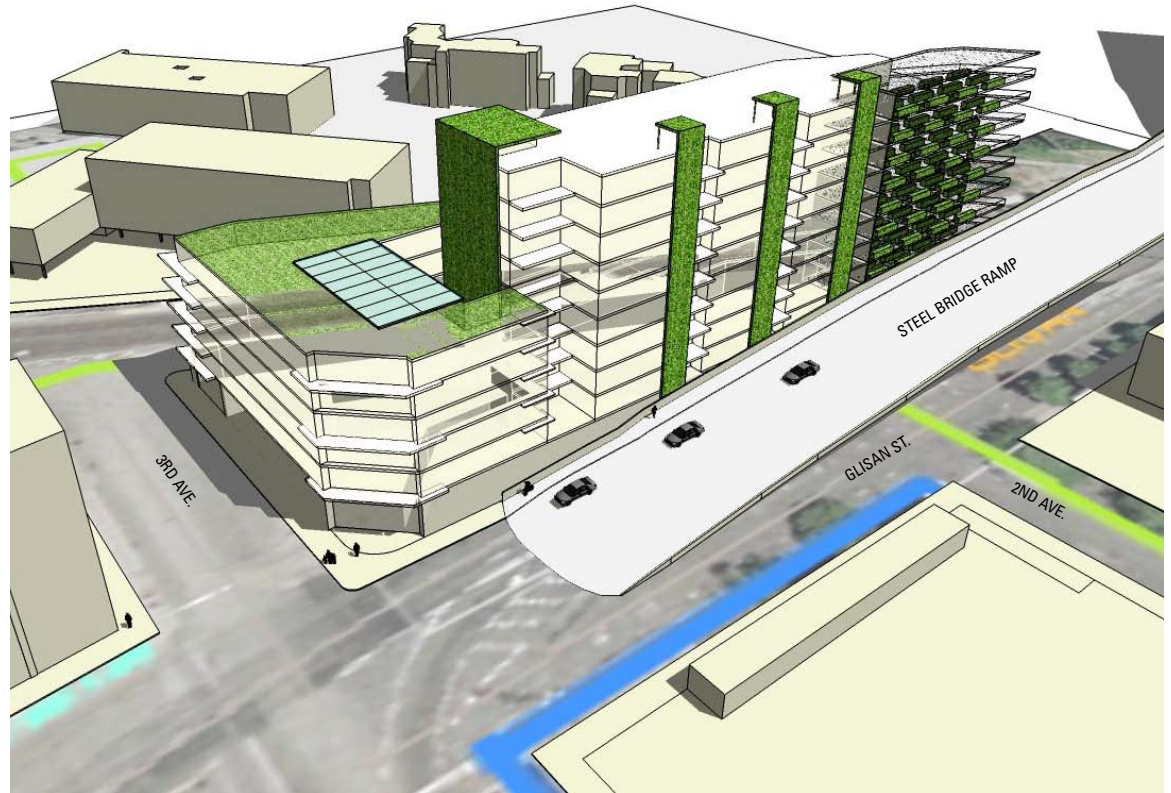
Aerial view from the southwest showing new construction over the full parcel. This would require removal of the Fire Station, which would allow for more efficient parking on the ground floor and mixed-uses above.
